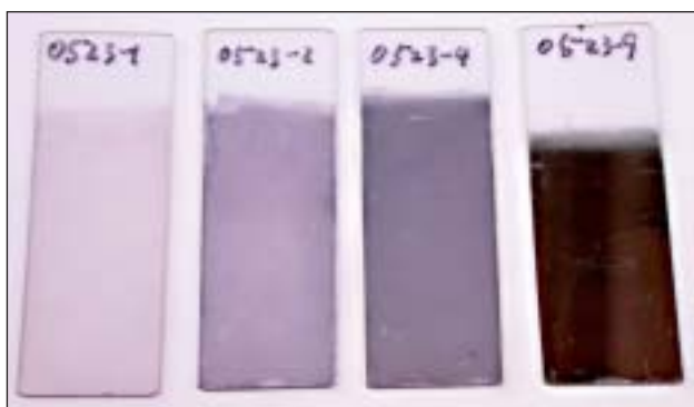
Figure 3 Glass slides that have been coated to varying extents with gold nano-particles, photo courtesy of Mr X. Xu, University of Technology Sydney
